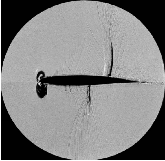
Fig. 10 Shadowgraph from two experiments, lower and upper sides; M_\infty = 0.74 and Re_c = 7.2 \times 10^6 .
